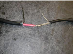
• Once the Red wire has been soldered to the coaxial cable wire, cover the joint with smaller heat shrink and use a heat gun to shrink and insulate the connection.
