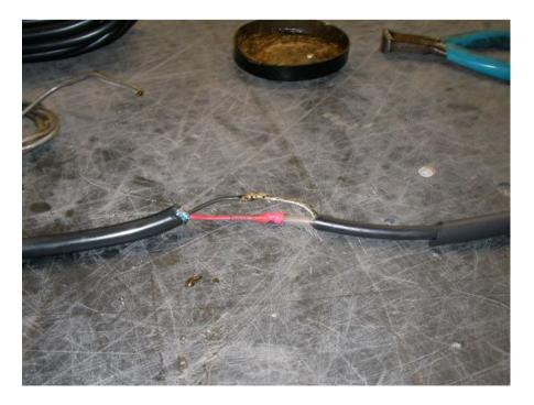
• Once the Red wire and Black wire have been soldered, cover joint with the larger heat shrink and use a heat gun to shrink and insulate the connection.
