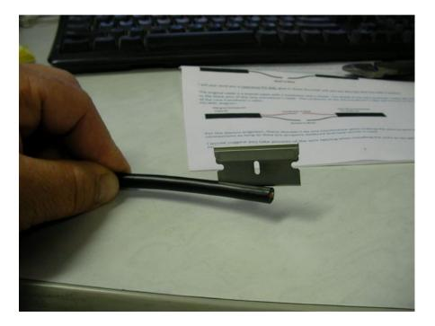
• Very carefully cut the black wire insulation off of each harness end without cutting into the internal wires present.
